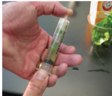
Figure 6a. Creating a Vacuum in the Plunger
